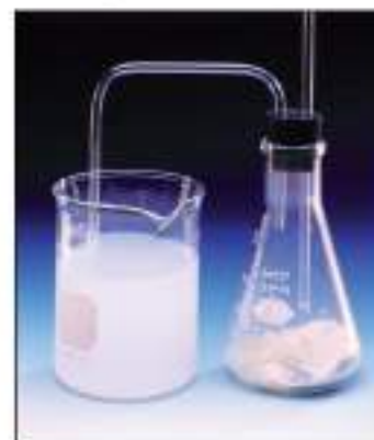
CO 2 turbids limewater
